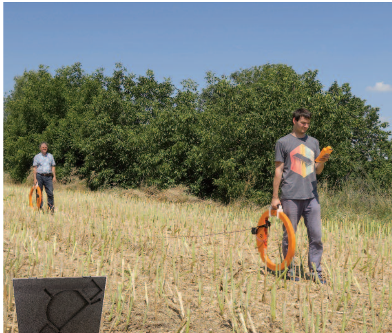
CMD - DUO single-depth, two-men operated probe with variable depth range 15 / 7.5 m or 30 / 15 m or 60 / 30 m for measurement of deeper situated structures (weathered zones, bedrock, cavities).
