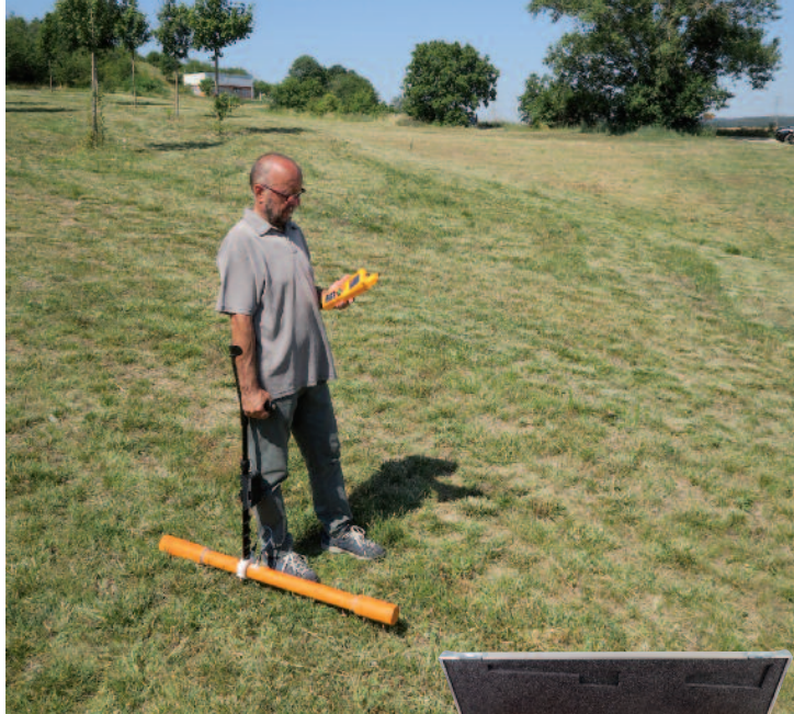
CMD - 1 economy single-depth probe with 1.5 / 0.75 m depth range for archeology, agriculture and buried metal object detection.
