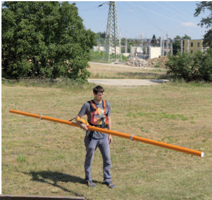
CMD-Explorer three-depth probe with depth ranges 2.2 / 1.1 m, 4.2 / 2.1 m, 6.7 / 3.3 m for extra wide range of applications with evaluation of vertical and horizontal conductivity changes.
