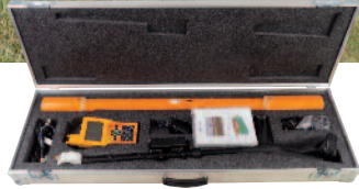
CMD - 1 economy single-depth probe with 1.5 / 0.75 m depth range for archeology, agriculture and buried metal object detection.
