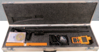
CMD - Tiny single-depth probe with 0.7 / 0.35 m depth range for assessment of very shallow objects in the frame of civil engineering, agriculture and archaeology.
