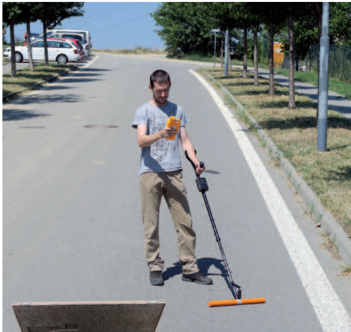
CMD - Tiny single-depth probe with 0.7 / 0.35 m depth range for assessment of very shallow objects in the frame of civil engineering, agriculture and archaeology.
