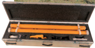
CMD-Explorer three-depth probe with depth ranges 2.2 / 1.1 m, 4.2 / 2.1 m, 6.7 / 3.3 m for extra wide range of applications with evaluation of vertical and horizontal conductivity changes.
