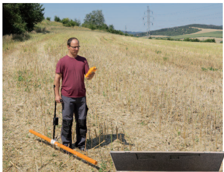
CMD-Mini Explorer 6L six-depth probe with depth ranges 0.3 / 0.15 m, 0.5 / 0.25 m, 0.8 / 0.4 m, 1.1 / 0.5 m, 1.6 / 0.8 m, 2.3 / 1.1 m for high resolution mapping and section imaging.
